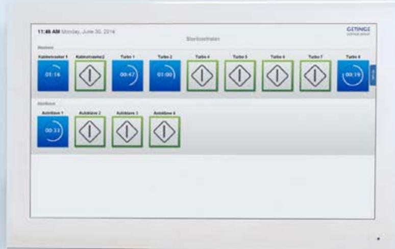
*Uncluttered information on an online monitoring screen enables viewing current equipment status, giving you full overview of remaining process time, alarms and warnings – without even having to go to a computer or the sterilizer.*
